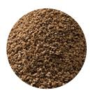
Ground walnuts shells are a type of abrasive blast media used for cleaning. The walnut shells are ground to various sizes from coarse to extra fine depending on the application. The walnut shells are used in the same manner as typical blast media. Walnut shells are durable and can be re-used in many applications. Walnut shells can remove matter from surfaces without scratching or pitting underlying material.
